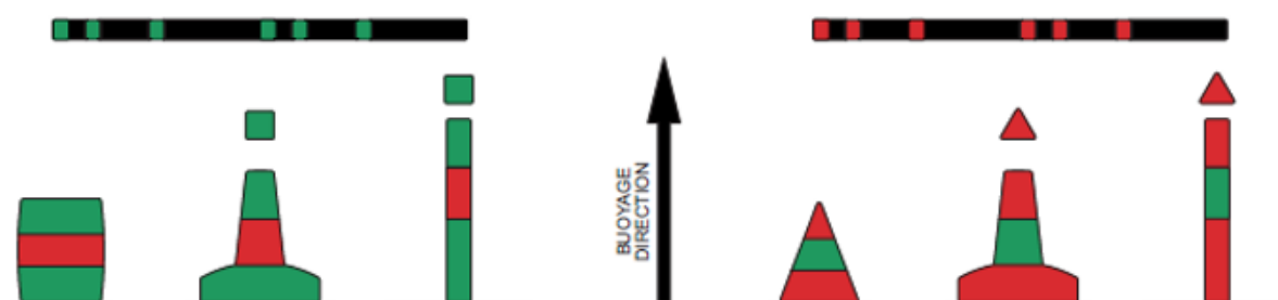
Figure 4 Preferred Channel marks used in Region B
